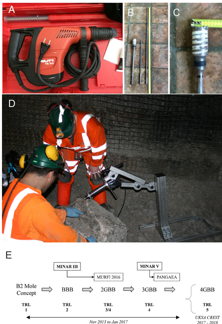
Fig. 4. Some of the sample acquisition instrumentation deployed in MINAR 5. (a)–(c) NASA drill. (a) The Hilti Drill TE 50, 1050 Watts; (b) 42 cm core string; 40.6 cm cutting string; 92.7 cm cuttings string; (c) core drill bit diameter 5 and 7 cm long, (d) The SPLIT instrument in operation on an artificial outcrop of halite in the Mars Yard; (e) the use of MINAR for the methodical development of the SPLIT technology (see ‘Results’ section for details).
